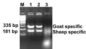
Duplex PCR for fiber identification: lane M 100 bp DNA ladder; lane 1: Sheep and goat blood DNA mixed in 1:1; lane 2: Sheep wool and Pashmina fiber DNA mixed in 1:1. Lane 3: Rabbit hair DNA. Sheep and Goat specific primers were used in all samples.
